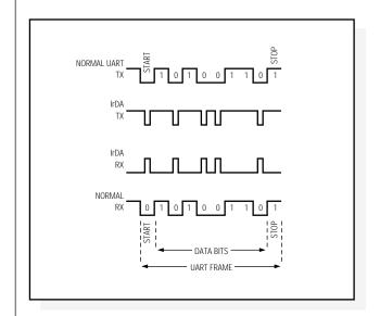
Figure 6. The narrow pulses used in IrDA communications consume less power.
