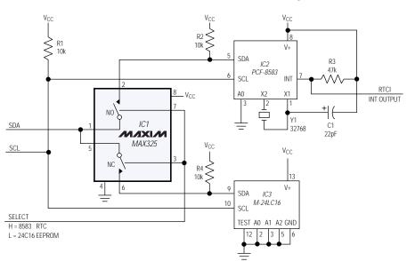
Figure 1. A dual analog switch (IC1) and a single controller line (SELECT) enable this I<sup>2</sup>C bus to select between two peripherals with identical addresses.
