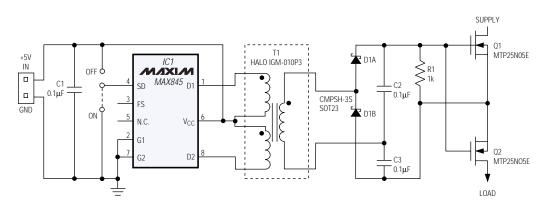
Figure 1. This bidirectional power switch handles moderately high positive, negative, and AC supply voltages.
