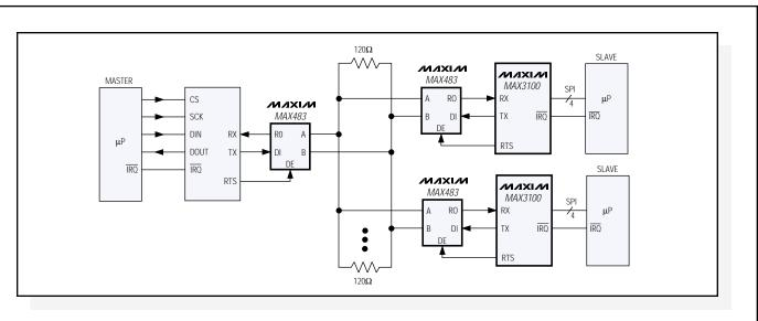
Figure 8. Nine-bit networks reduce the processing overhead in a communication network.
