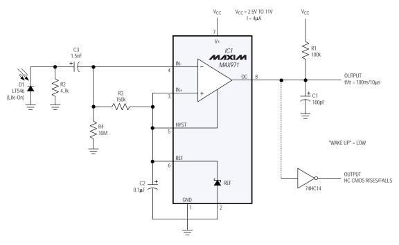
Figure 1. This low-quiescent-current circuit (4µA maximum) interrupts the host processor when it detects an IR signal.
