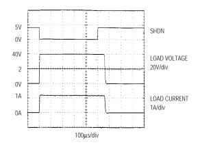
Figure 2. This scope plot shows the Figure 1 circuit operating with a 40V, 1.2A load.
