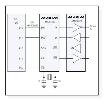
Figure 7. The MAX3100 enables IrDA communications by variants of the 8051 microcontroller.
