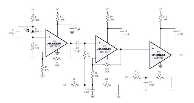
Figure 1. These two op amps and comparator form a tiny photodiode receiver for data rates to 800kbps.
