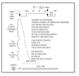
Figure 2. These details show how the CPU time is allotted in servicing a software UART.
