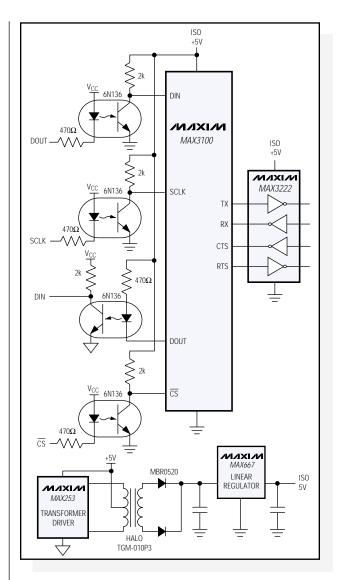
Figure 9. MAX3100 I/O pins are designed for a direct interface to optocouplers.
