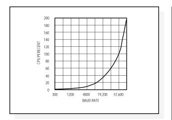
Figure 3. The percentage of CPU time required for servicing a software UART rises sharply with the baud rate.
