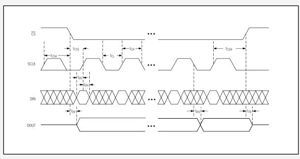
This SPI serial-interface timing is closely related to that of the QSPI and Microwire standards.
